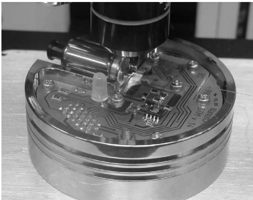
FIGURE 1.2 (Color figure follows p. 12.) Photograph of miniature STM mounted on the Raman microscope stage.
