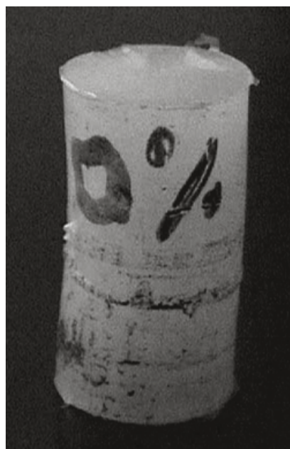
FIGURE 17.4 Cylindrical polypropylene neat resin specimen after compression testing.
