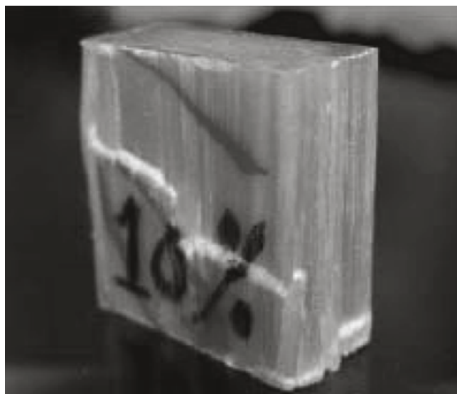
FIGURE 17.5 Pultruded compression test specimen (10% nanoclay loading) after failure.
