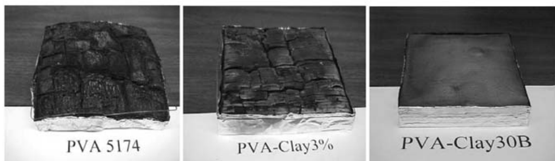
FIGURE 16.10 Digital photos of combustion residues of wood blocks coated with PVA 5174 (left), PVA– 3% MMT clay (center), and PVA–30% MMT clay (right).
