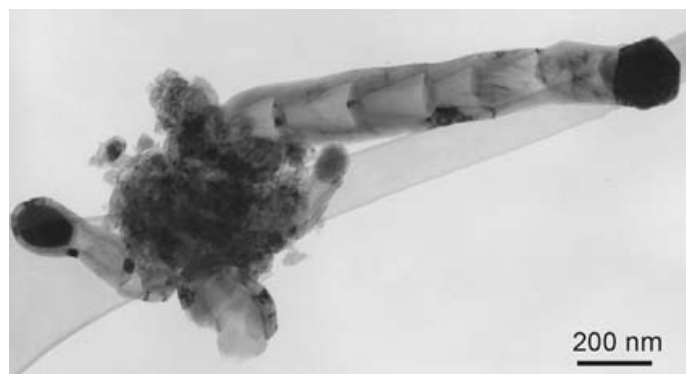
FIGURE 7.19 TEM image showing BN nanotubes with bamboo-like structures, which formed in the BN samples after first milling, and then subsequently heated at 1200°C for 16 h. The dark particles at the tips are Fe. 15
